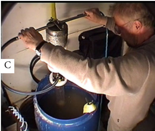
Figure 9. The AKUT vibracorer on test in dry soil (A, B) and an artificial seabed (C, D). Photos AKUT
