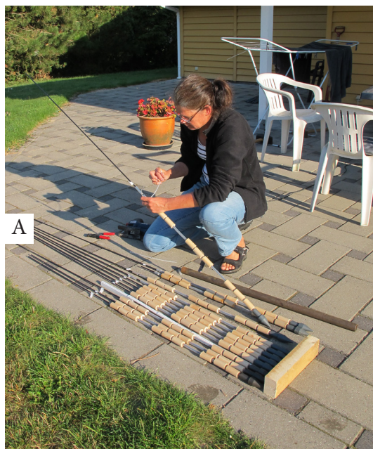
Figure 16. Dr Charlotte Björdal from the University of Gothenburg preparing modern wood samples (A). On each kebab there are two sets of samples that are buried within the sediment and one set of samples exposed to the open seawater as a negative control. (B). Photos National Museum of Denmark.
