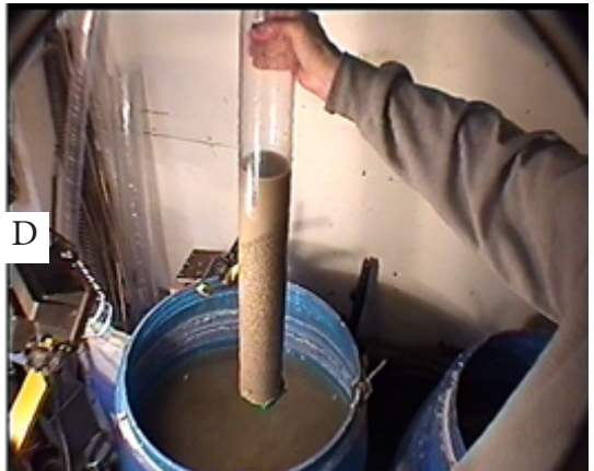
Figure 9. The AKUT vibracorer on test in dry soil (A, B) and an artificial seabed (C, D). Photos AKUT
