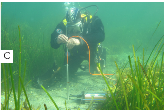
Figure 15. The microsensor with hypodermic needle which is passed into the metal spear and passes through the septum into the sediment (A). End of the spear with the hypodermic needle of the microsensor passing through (B). Inserting the microsensor into the spear (C). Waiting for the sensor to stabilise (D). Photos Viking Ship Museum.
