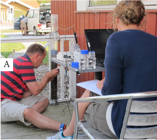
Figure 14. Dr Mikkel Holmen Andersen (Unisense) and Anne Marie Eriksen (National Museum of Denmark) measuring sediment profile parameters in the cores (A). Set up for measuring profiles. The plastic core tubes had silicone filled holes drilled into them every 5 cm, enabling a microsensor to be passed through and the parameters measured (B). Photos National Museum of Denmark.
